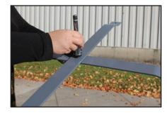
Align the holes in the middle of both cross base arms and insert the flag spindles into the hole from the top. Twist the spindle until it securely holds the two arms together.
