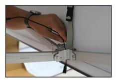
After positioning all four LED light strips in their desired locations, run the spiral power cord along the scissor piece to the outside frame. Feed the cord through the opening in the scissor piece joint and run to the frame corner of your choosing.
