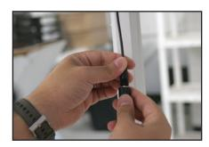
Attach the power cord plug and remainder of power cord by twisting the power cord socket into the LED light band cord socket.
