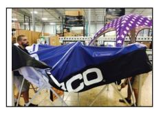
Confirm peak grommet and canopy corners are properly attached to the tent frame. Expand the tent frame by pulling on opposite sides of the tent frame legs.
