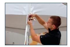
Once the lid is secure, feed the end of the bottom strap up into the ratchet that is located at the bottom end of the top strap (this is the strap installed in step 2).
